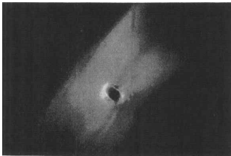
Figure 8. Disclination loop in capillary; crossed polarizers, approx. 32\times .
